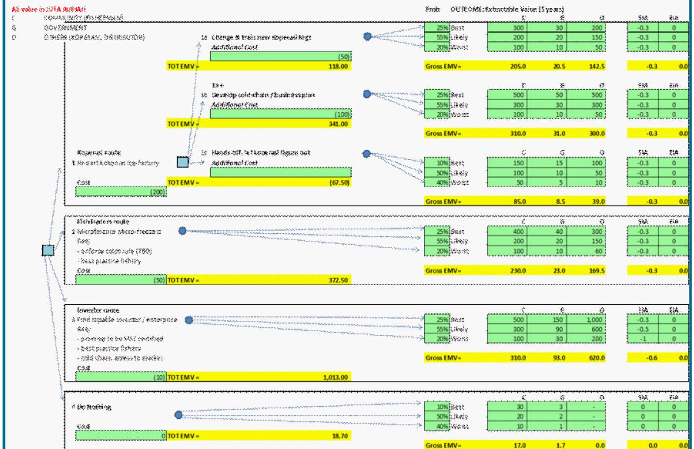
Fig. 6.4: Decision Tree for analyzing the benefit of three cold-chain development options in Mimika
